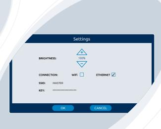
Adjust the brightness on the controller display and choose the most convenient type of connection to the local network, wirelessly over Wi-Fi or with an Ethernet cable.
